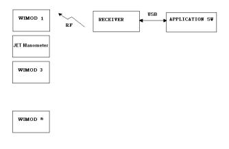
The first level is the communication between the application sw and the receiver RF module.
